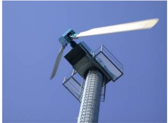
The pressure of the wind pushes the blades in the direction of the main shaft. Due to the hinges in the rotor hub, the actual position of the blades will be slightly backward. Instead of a disc perpendicular to the main shaft,
